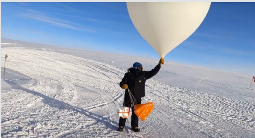
Figure 1 A scientist launches a weather balloon carrying an ozonesonde from South Pole Station in March of 2021. Credits: NOAA Global Monitoring Laboratory.
